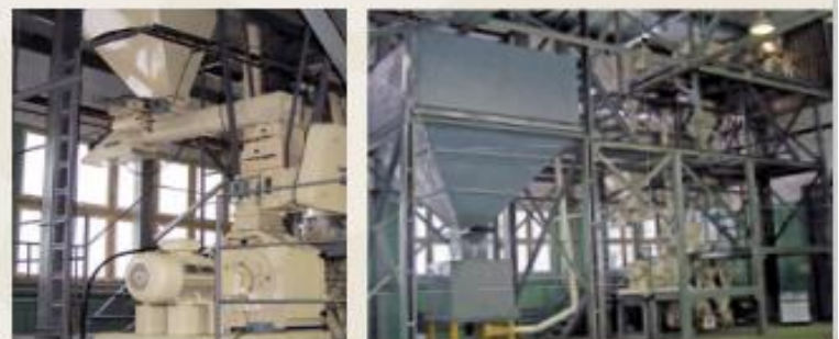
ALLIGNO, MOSCOW, RUSSIA - VDK 4.1 ATEX HAMMER MILL DESIGN (ENTRY INTO SERVICE 2007) - WOOD GRINDING: 0.8 T/H (1.0 MM FILTER) FINE GRINDING FOR WPC PRODUCTION 99% < 0.7MM
