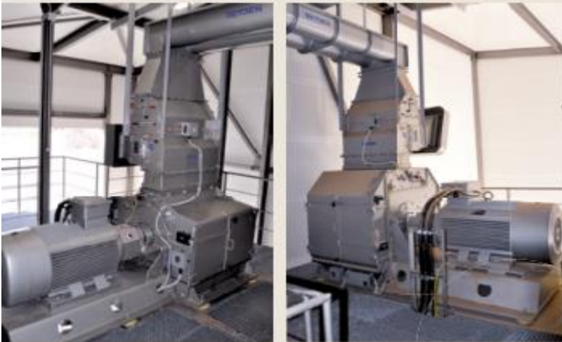
PELET GRUPA, NOVSKA, CROATIA - W 1000 WIDE CHAMBER HAMMER MILL (LEFT) (ENTRY INTO SERVICE 2014) - WET WOOD GRINDING: 12 T/H CHIPS UP TO G50 (15MM FILTER) FOR FURTHER PROCESSING ON THE DRYING LINE - GD 25 HAMMER MILL (RIGHT) (ENTRY INTO SERVICE) - WOOD GRINDING AFTER DRYING: 6 T/H (6MM FILTER) FOR PELLET PRODUCTION 99% < 4 MM
