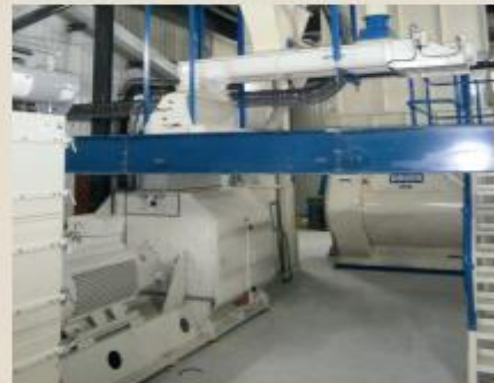
Montego Site in South Afrika: Preparation of compounds for Petfood. GD 25 Module with Plansifter (Grinding concept V1)
