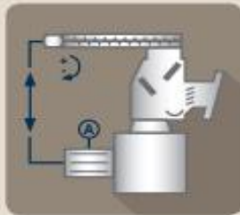
Load dependent dosing of the raw material into the grinder
