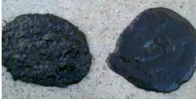
Fermentation substrate: More flowable due to IMPRA (left before, right after digestion)
