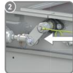
Pneumatically operated inlet flap (optional)
